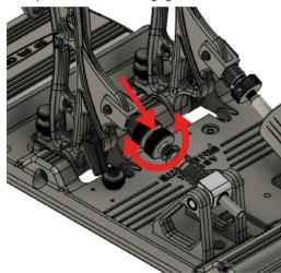
3. Turn the uppermost thumbnut counterclockwise to retighten it, locking the bottom thumbnut in its position.
