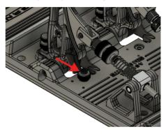
3. Re-tighten the thumbnut by rotating it clockwise.
