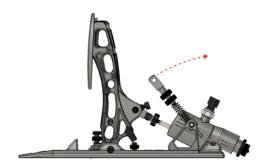
3. Push the pedal slightly forward and rotate the thumbscrew (Clockwise to move the pedal forwards, Counter-Clockwise to move the pedal backwards)
