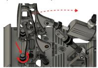
4. Once you have achieved your desired position, tighten the locking thumbnut and re-insert the rod clevis
