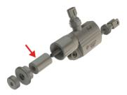
5. Grab the larger thumbnut and turn it onto the shaft clockwise until you reach your preferred setting (see 4.2.10 brake pedal preload adjustment).
