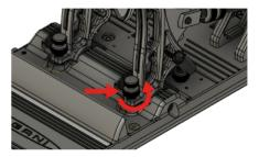
2. Remove the rod clevis and lift up the rod
