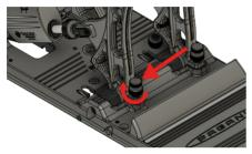
7. Adjust the pushrod length by turning the clevis until it perfectly matches up with the hole in the pedal arm. Reinsert the clevis lock pin.
