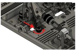
2. Use an Allen key to adjust the height of the Allen screw.
