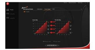
As we briefly mentioned, a real race car will not have a linear throttle response. An example will be an Audi R8 LMS GT3, which has less activation of the throttle at the beginning of the pedal activation, increasing as you progress through the travel. Similarly, you can adjust your curves based on your driving conditions—all in search of ultimate performance.
