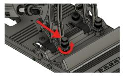
5. Push the pedal slightly forward, and rotate the thumbscrew
